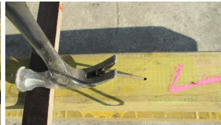
Correct method of removing nails
