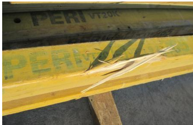
Damages caused by nails
